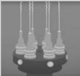
The SNC Fibers story began with a prototype improvement on traditional nanofiber spinning technology, in which nanofibers are spun from an electrically charged injector needle, through which a polymer is injected onto an electrode plate.
